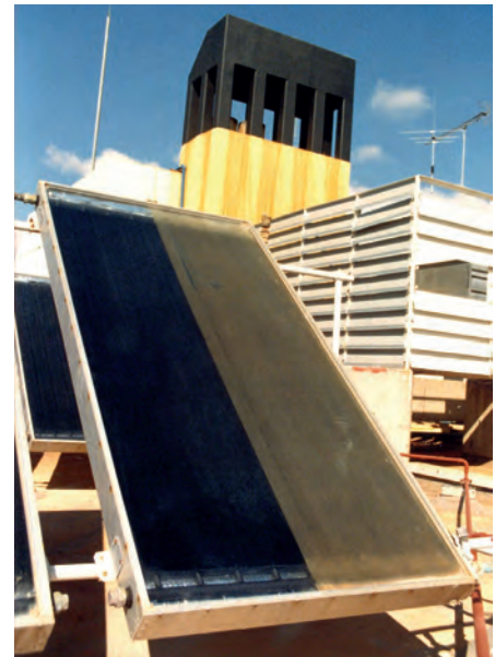
A solar panel, half treated with Ritec's ClearShield.
